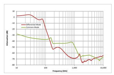
Figure A: Typical Common Mode and Differential Mode Attenuation provied by the filter as a function of frequency. Source resistance is  $50\Omega$ .
